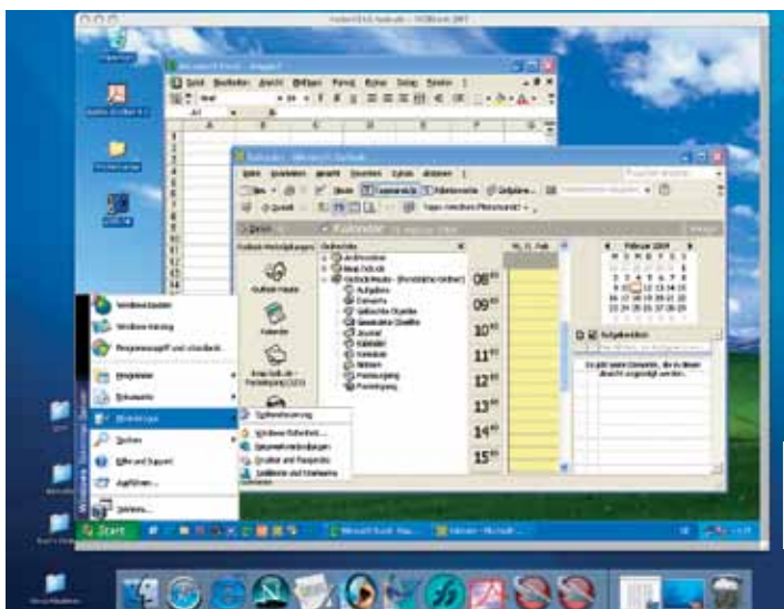
HOBLink JWT – the Java client for Windows Terminal Servers – here on a Mac OS X desktop.
